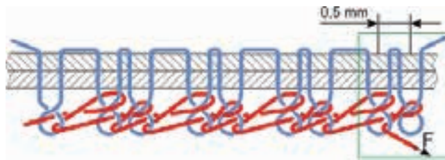
Special new non-ravelling, high breaking strength chain seam, where every normal chainstitch has one normal chainstitch with a length of 0.5 mm as bartack
